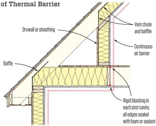
Air-sealing needs to be part of the framing stage; it's not something that can be done as an afterthought. Knee walls are one of the framing locations where it's often done wrong. The best way to handle them is to move the thermal barrier to the roofline and stand up the knee walls after the ceiling has been drywalled. For production builders who may have less control in scheduling trade partners, the knee wall can serve as the thermal barrier, as long as sheathing is installed on the back side.
