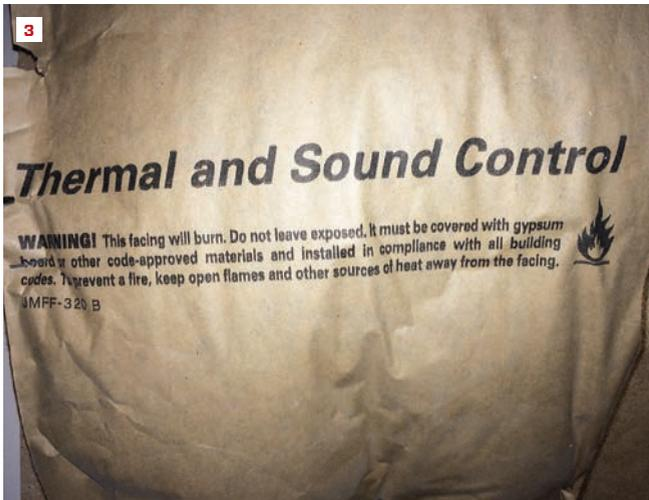
The warning label on paper-faced insulation batts clearly states: "This facing will burn ..." It cannot be left exposed but must be covered with drywall or other type of sheathing permitted by code. This applies in concealed framing cavities, in knee-wall areas (even if the knee-wall area is inaccessible) in attics, and in crawlspaces.
