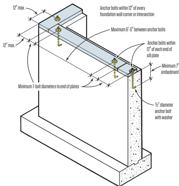
Given the anchor-bolt requirements (these conform to the 2012 IRC), it’s often easier to use epoxy anchors. J-bolts require coordination between framing and concrete crews.
