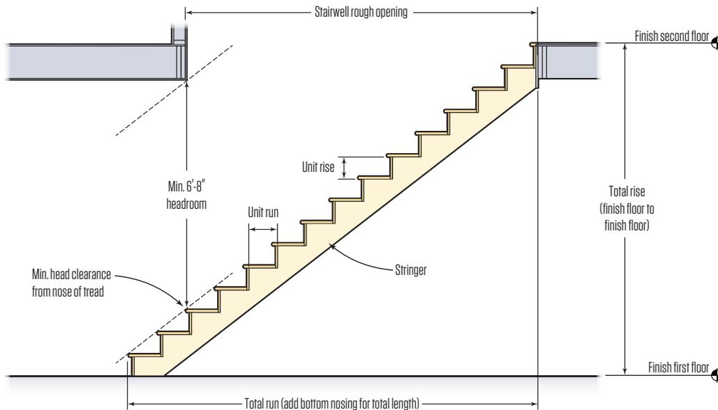
Headroom is often the limiting factor for a given stair opening. Building codes require a minimum 6 feet, 8 inches from the tread to the ceiling. Shortening the stairs only works if you can maintain tread and riser requirements. The steepest residential stairs allowed by code has 7 <sup>3</sup>/<sub>4</sub>-inch risers and 10-inch treads.
