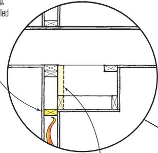
If drywall has been installed on the wall before the soffit is built, no additional fire blocking is needed
